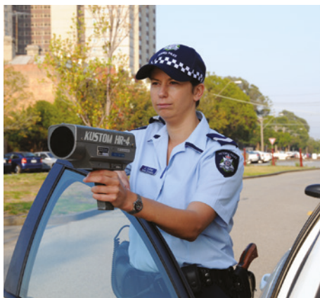
FIGURE 11.2.2 To avoid a systematic error, make sure that you are using measuring equipment correctly. Laser speed guns, for example, need to be placed on a stationary support so the aim point is held on a single target point for the duration of the read.
