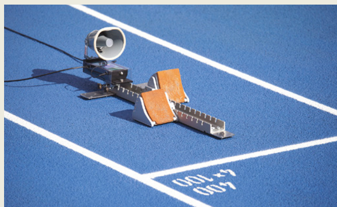
FIGURE 7.1.4 Starting blocks are fitted with pressure sensors to detect false starts.
