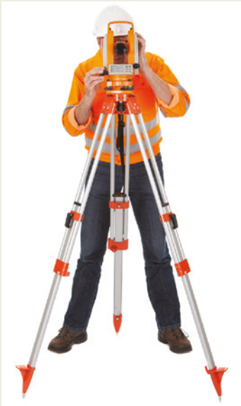
FIGURE 6.2.8 Surveying the land with a theodolite.
