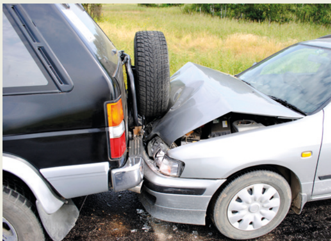
FIGURE 8.6.5 The crumple zone on this car has prevented serious damage to the car's occupants.
