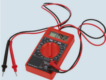
FIGURE 5.3.8 A digital multimeter can be used as either an ammeter or a voltmeter.
