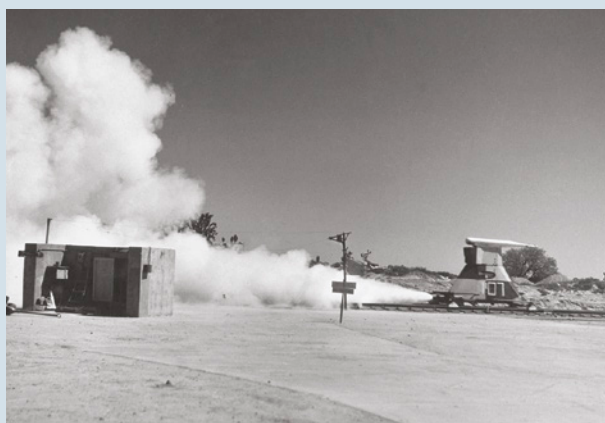
FIGURE 7.2.3 The rocket-powered sled used to test the effects of acceleration on humans.
