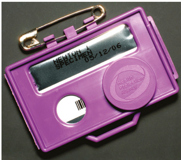
FIGURE 3.5.5 Thermoluminescent dosimeters are used by doctors, radiologists and scientists who work with radiation to monitor their exposure levels.
