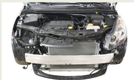
FIGURE 2.4.5 A radiator is often placed at the front of the car where it can take advantage of the airflow over the moving car.
