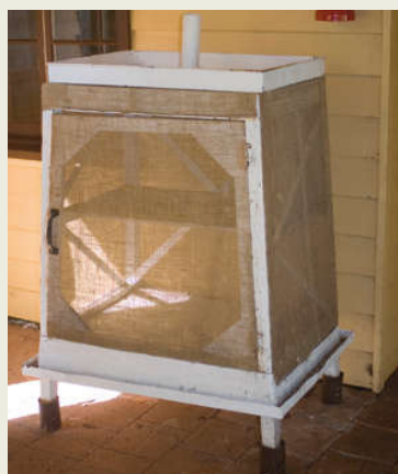
FIGURE 1.3.3 Early model of the Coolgardie meat safe.
