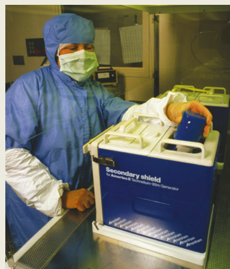
FIGURE 3.2.8 Technetium generators are used in hospitals that require radioisotopes. The generator has a thick lead shield that absorbs the beta and most of gamma radiation.
