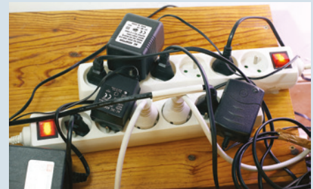
FIGURE 5.6.6 Overloading of power boards.
