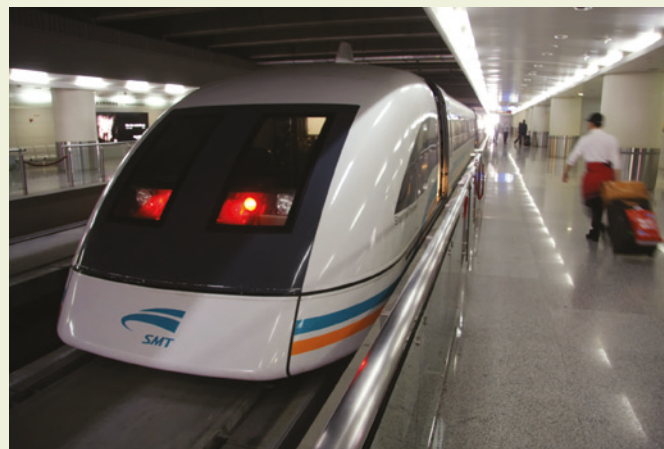
FIGURE 8.3.8 This magnetic levitation train in China rides 1 cm above the track, so the frictional forces are negligible. The train is propelled by a magnetic force to a cruising speed of about 430 \text{ km h}^{-1} .
