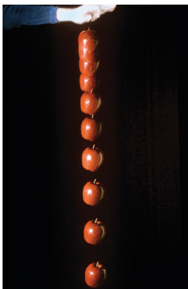
FIGURE 7.5.1 A stroboscopic image of a free-falling apple. The time elapsed between each image of the apple is the same but the distance it travels increases, which shows the apple is accelerating. Without air resistance, this rate of acceleration is the same for all objects.
