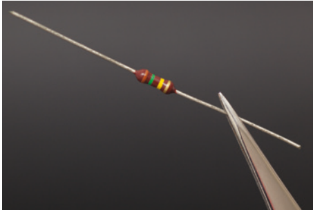
FIGURE 5.4.7 Common resistors are electrical devices with a known resistance. The coloured bands indicate the resistor's resistance and tolerance.
