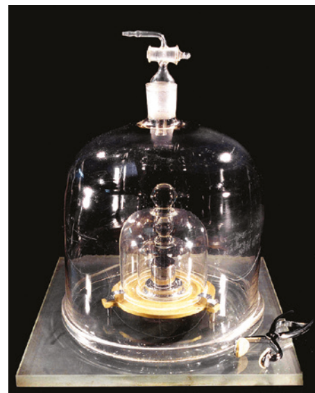
FIGURE 8.7.1 All mass in the world is compared to this small piece of platinum–iridium alloy held in a sealed vault in Paris.
