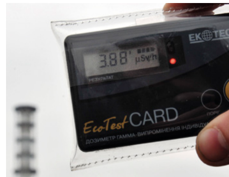
FIGURE 3.5.1 A dosimeter used to monitor gamma radiation exposure.
